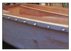
Rubbing beads are glued and screwed. When set the screws are removed and the holes plugged making a nice row of cannon ports!!! (until faired off)
